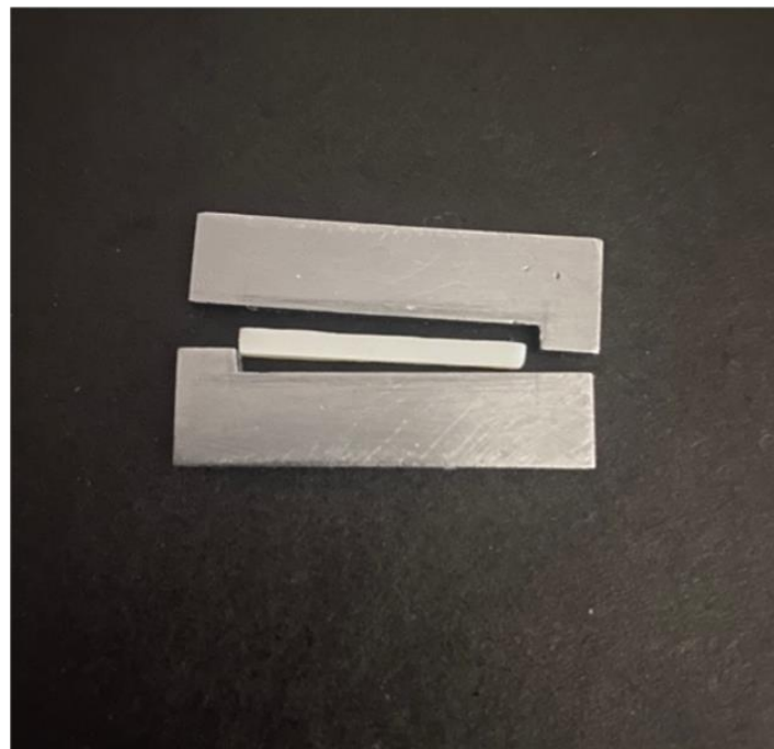
Figure 2. The sample is removed from the matrix after polymerization.
